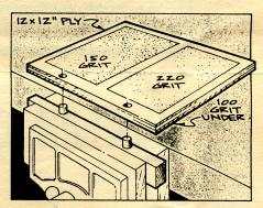
the board allow it to be held by the cleat. This also enables me to use sandpaper on both sides of the board. I use a full sheet of 100-grit sandpaper on one side and half sheets of 150- and 220-grit on the other.
