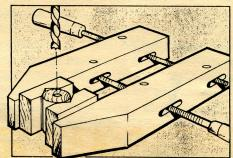
stock. Also, if you cut the V-groove square to the bottom edge of the block, the V-block will align the stock square to the drill-press table.
