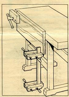
need to support a long board at the workbench. One hand screw clamped to a piece of scrap stock serves as the base, while a second hand screw, clamped at the proper height, supports the board.
