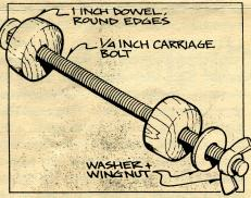
carriage bolts (fully threaded), and 1/4 in. washers and wing nuts. They are great for any job where you need to apply light clamping pressure near the edge of your stock.
