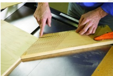
A proper featherboard. The fingers of a featherboard are consistent in size and springy, as shown. You can clamp them to the table or to the fence to help im-
